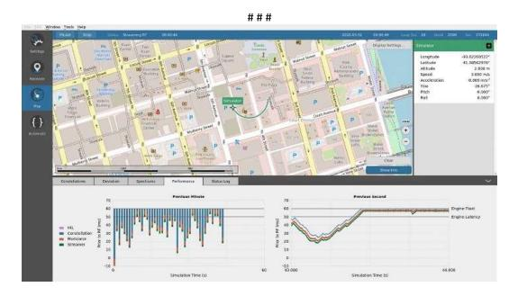
"The Orolia Skydel Real-Time Performance graphs illustrate the software-defined engine's low latency during a GNSS simulation."
